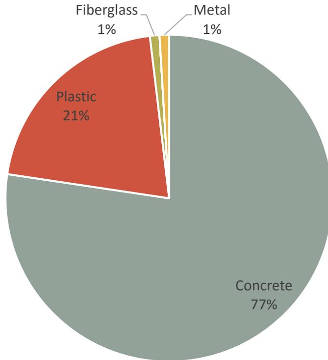
As a result of the re-inspection program, it was noticed that **18.8%** of concrete septic tanks had signs of corrosion (Illustration 1). Concrete corrosion can be caused by a build of gases (from normal operation) reacting with the concrete. The corrosion can cause baffles to fall off, effluent to escape around the outlet pipe and the tank to become structurally unsafe.
