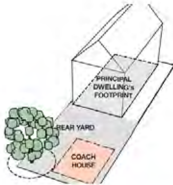
Figure 4 Detached ARU (source: City of Ottawa)
